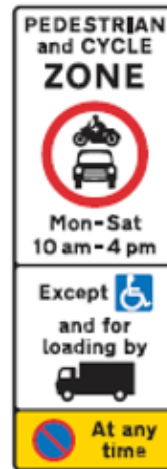
Figure 6-2 Diagram 618.3C (S8-2-2) Entry to, and waiting in, pedestrian and cycle zone restricted
